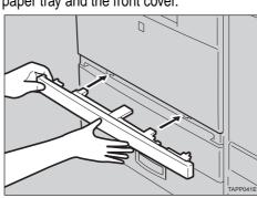
To install the paper bank PS430, see "Installing the Paper Bank PS430" in the "Operating Instructions".
