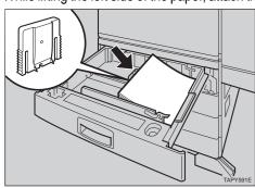
Slide the tray into the printer until it stops.
