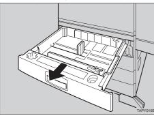
Pinch the sides of the rear guide (1), and remove it (2).
