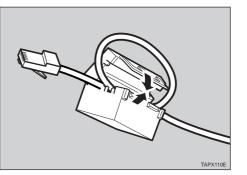
Attach the network cable to the network cable connector of the printer. Secure the cable.
