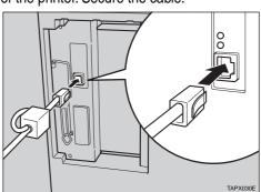
Connect the other side of the cable into the network. Secure the cable
