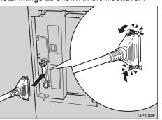
Attach the other end of the parallel cable to the parallel interface connector of the computer. Secure the cable.
